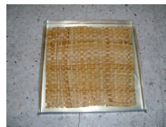
Figure 13 Pseudo-stem banana Fiber reinforced epoxy composite during the curing process
