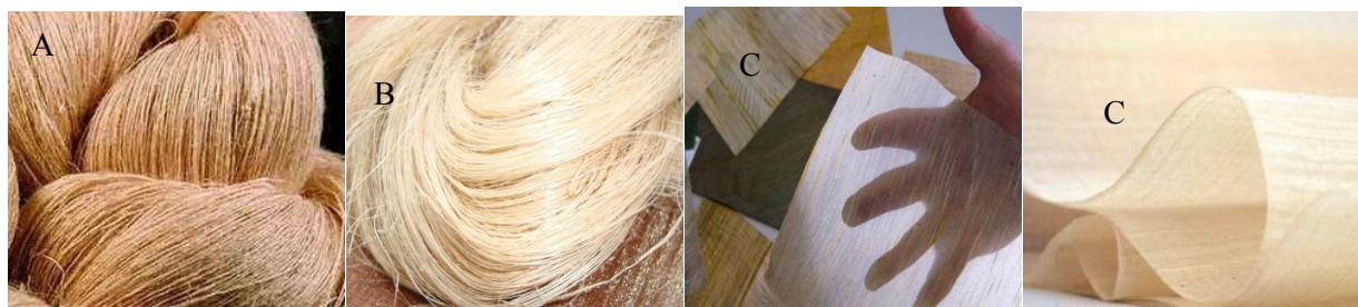
(A) Coarse(rough) Fiber (B) Fine and smooth fiber (C) banana fiber fabric silk looks like Figure 6 Types of Banana Fiber
