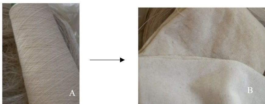
Figure 7 (A) Banana spun yarn (B) Banana fiber knitted trial
